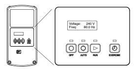
The DC2 controller provides integrated control for the generator set, Kohler® Model RXT transfer switch, programmable interface module (PIM).
